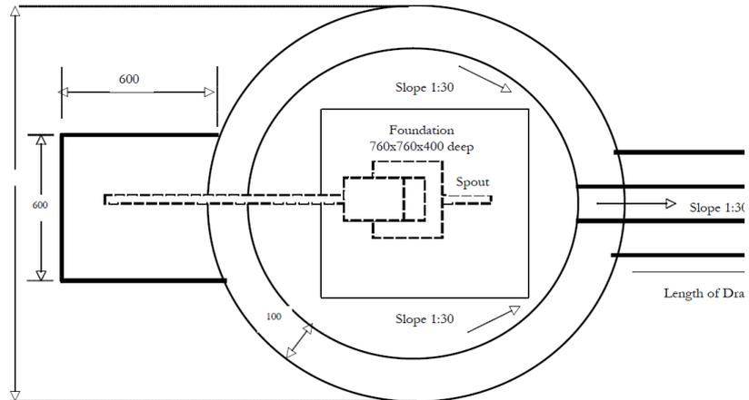
**Figure 5: A U3M pump on a sealed borehole with concrete apron**
