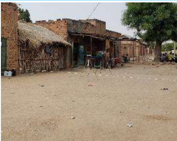
Aeroqual S500 Monitor placed on a tripod stand 1.2m above the ground in Nakibengo TC
