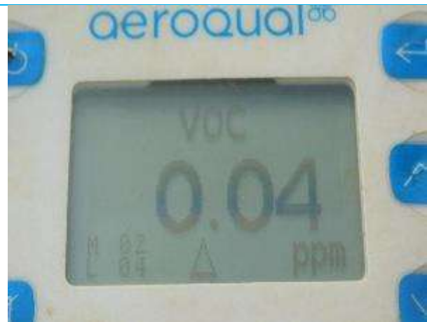
Display of results by Aeroqual S500 Monitor during measurement of ambient air quality
