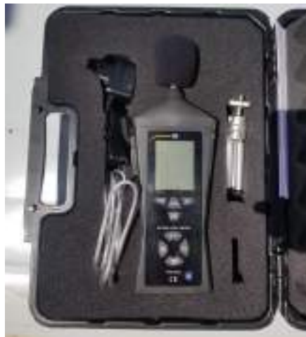
Figure 2-2: PCE-322A sound level meter
