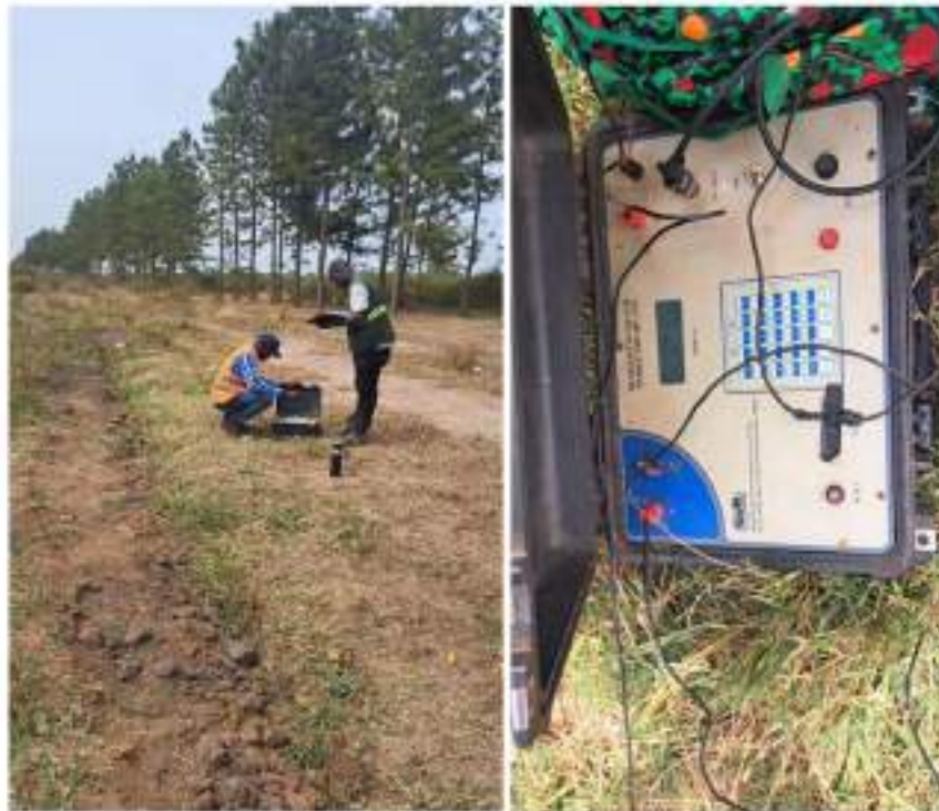
Figure 7: Resistivity test at the treatment point
