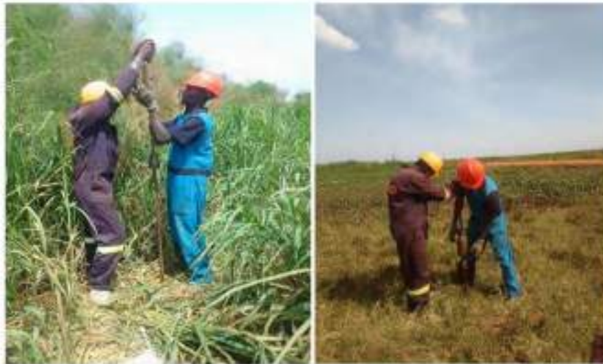
Figure 6: Photos showing Dynamic Penetrometer Tests in Progress
