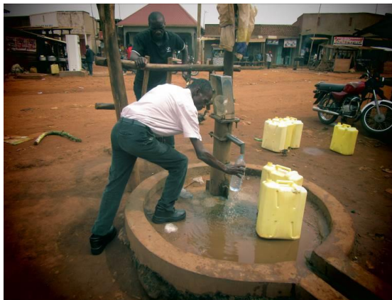
Plate 2: Obtaining a water sample from the existing borehole
