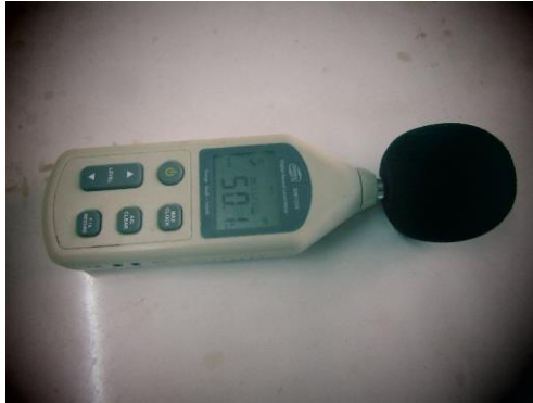
Plate 3: Noise level meter used for noise assessment
