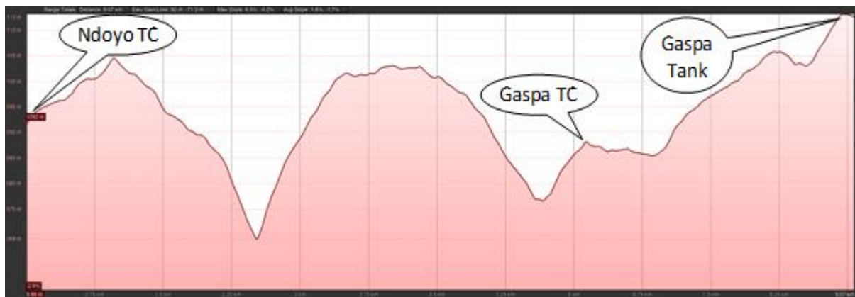
Figure 5-19: Elevation profile of the Water pipe line for distribution lines of Gaspa RGC
