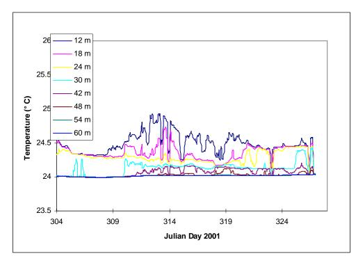
FIG. 5. Temperature profiles for station UP8 November – December 2001.
