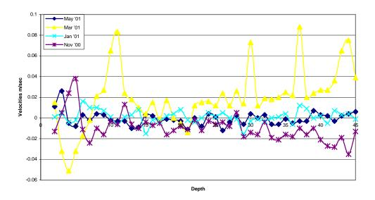
FIG. 12. Vertical velocities for UP6 at selected times of the year.
