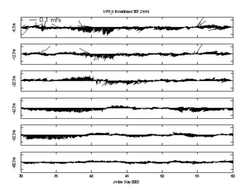
FIG. 15. Velocities at UP8 measured from January to April 2002.
