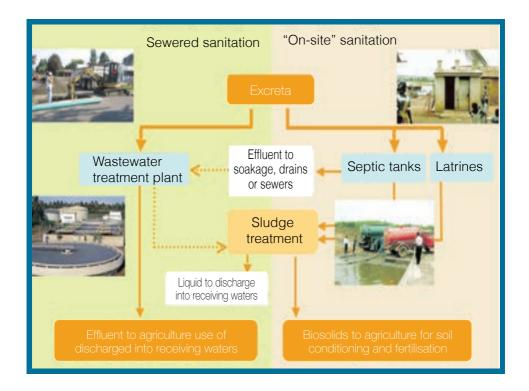
Figure 5-1: Faecal sludge and wastewater management side-by-side in urban environmental sanita-tion and their potential links Source: Adopted from Eawag/Sandec, (2008)
