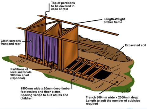
Figure 26: Typical design and layout of a trench latrine
