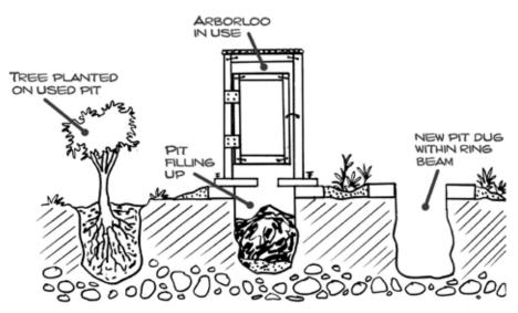
Figure 29: Schematic Diagram of an Arborloo
