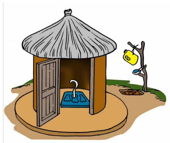
Figure 27: Typical traditional pit latrine improved with SanPlat
