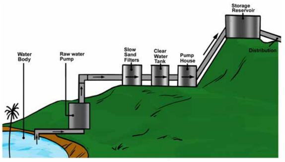
Figure 20: Diagrammatic representation of a piped water supply system
