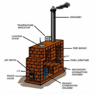
Figure 48: Typical layout of double combustion chamber incinerator
