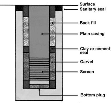
Figure 14: Tube well design and installation
