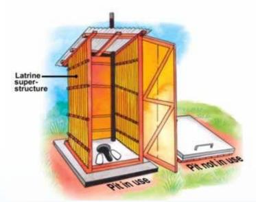
Figure 31: A typical layout of the Fossa Alterna toilet
