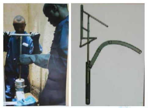
Figure 38: The Gulper I in use (left) and the Gulper II (Rammer Model)
