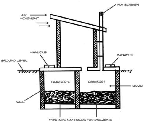
Figure 33: Alternating pit with two chambers
