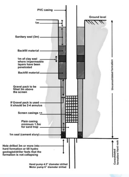
Figure 15: Detailed outline design and installation of borehole
