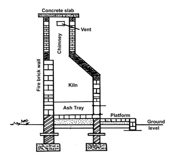
Figure 47: Typical single combustion chamber incinerator
