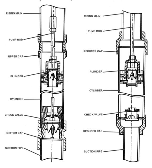
Figure 17: Cylinder assembly for U3 (left) and for U2 (right)
