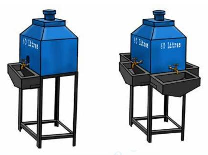
Figure 45: HWF with multiple taps (left) and with a single tap (right)
