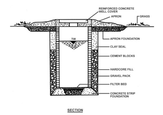
Figure 13: Section through a hand dug well
