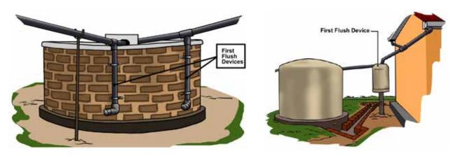
Figure 7: Small capacity FFD (left) and large capacity FFD with washout valve
