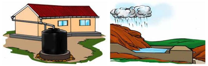
Figure 2: Roof catchment (left) and rock catchment rainwater harvesting system
