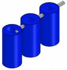
Figure 37: Pour flush latrine with barrels as septic tanks
