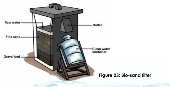
Operating the filter is very simple. Remove the lid, pour a bucket of water into the filter, and immediately collect the treated water in a clean container. The operating guideline is usually provided by the manufacturers to make sure filter produce water of acceptable quality.
