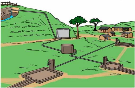
Figure 19: Schematic presentation a gravity flow scheme
